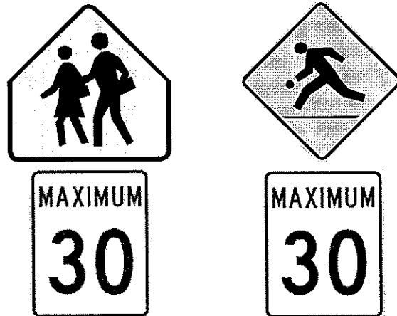
WC-1 and RB-1 (School Zone)
